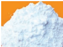
Calcined Shell Calcium created at over 1,100°C (2,012°F)
